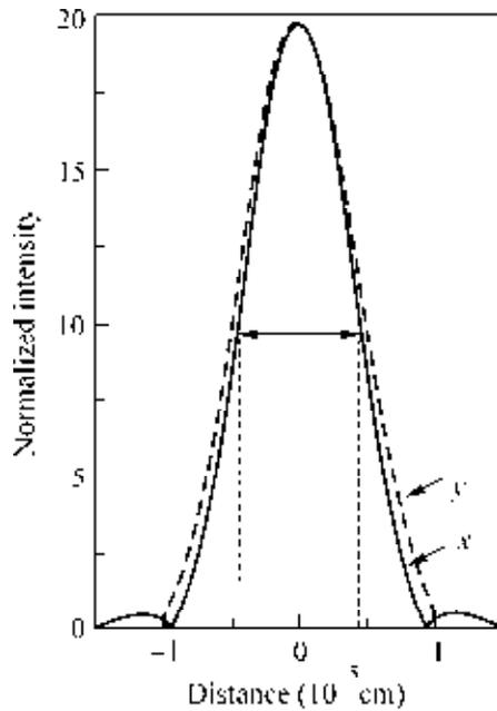
**Fig. 3.** The light intensity distributions ( $z$ -component of the averaged Poynting vector) on the substrate surface under the spherical particle (calculations with the Mie theory). Vector  $\mathbf{E}$  of the incident plane wave is directed along the  $x$  axis, vector  $\mathbf{H}$  along the  $y$  axis. Distribution of the surface intensity along the  $x$  axis is shown by a solid line and along the  $y$  axis by a dashed line.
