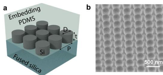
**Figure 1** (a) Schematic of the dielectric metasurface consisting of an array of silicon nanodisks on top of a fused silica substrate and embedded into a PDMS layer from the top to realize refractive index matching. (b) Example of the fabricated nanodisk array: tilted view ( $52^\circ$ ) SEM image, showing good uniformity, edge profile and approximately 90-nm interparticle gaps.
